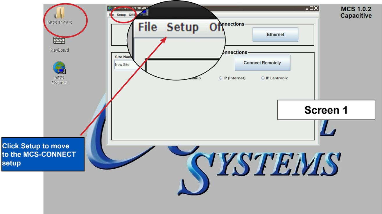
3. Next screen is the setup screen for communicating with your controller or PC.
